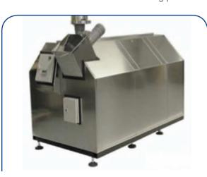
Dewaterer by gravity feed from the Food Waste Disposer. Excess liquid is pressed out and discharged to the drain whilst the residual solid fraction, ie "dry" waste, is expelled from the chute and collected.
